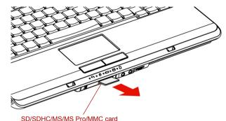
Figure 8-4 Removing the inserted memory card
